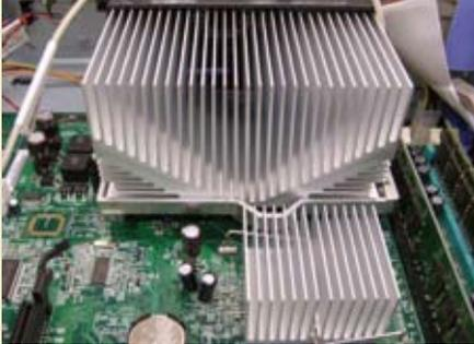
Heat sinks used in PC dissipate heat efficiently by using a large surface area to volume ratio.
