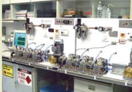
A self-developed testing to simulate the wear condition of artificial finger joints.
