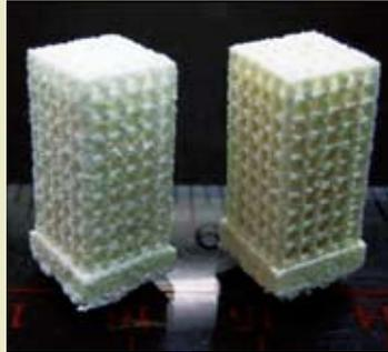
Nano-composite scaffolds for bone tissue engineering made from a selected laser sintering process.
