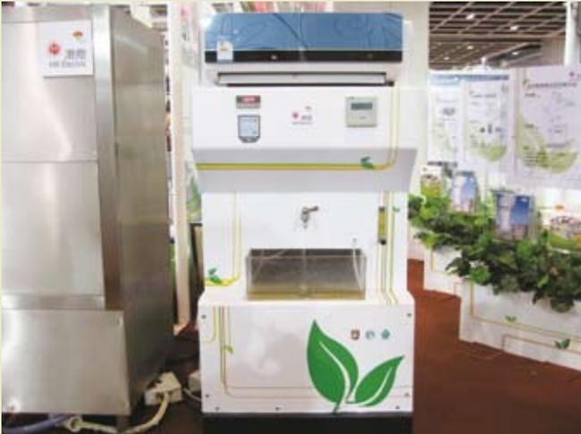
In large hotels, heat pumps are installed to extract the heat dissipated by air-conditioning systems to warm up tap water for sanitary use. The photo shows a small heat pump designed by our department under the sponsorship of Environment & Conservation Fund and Woo Wheelock Green Fund. The heat pump can be adopted in residential flats in which split-unit air-conditioners are used.
