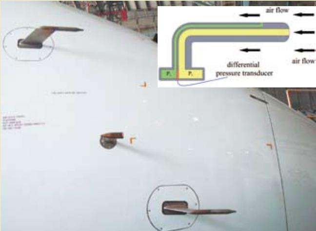
Pitot-static tubes equipped in a jetliner for flight speed measurement.
