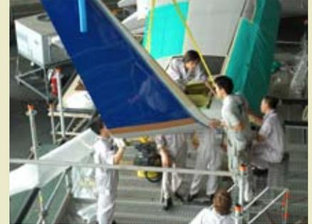
Winglet modification on a Boeing 737 aircraft. (Courtesy of HAECO).
