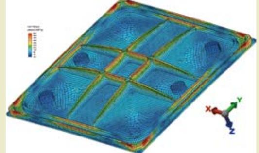
Stress analysis for a Class B-125 kN manhole cover. (Courtesy of Dextra Pacific Ltd)
