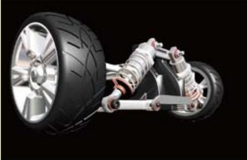
Pneumatic tyres, springs and hydraulic dampers are commonly used in the suspension system of road vehicle. (© Kristy Pargeter | Dreamstime.com)
