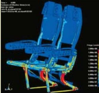
Our Department conducted computational analyses of an aircraft cabin seat for Hong Kong Productivity Council. The figure shows the stress level when the seat is undergoing 16g deceleration.
