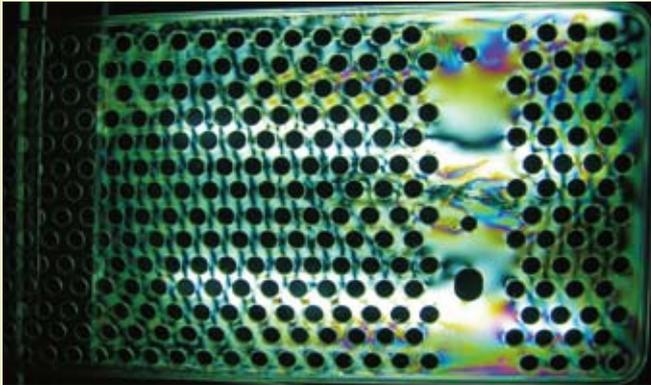
Photoelastic method is used to assess the residual stress, which can be visualized in the form of colourful fringes, in a polycarbonate panel. (Courtesy of Architectural Acoustics)
