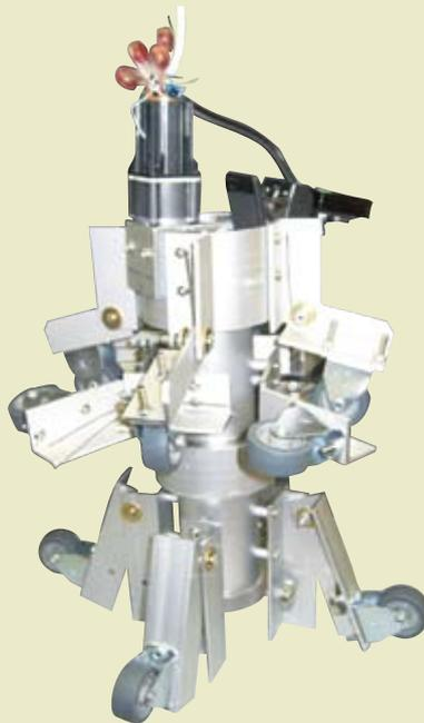
To extend the service life of underground pipelines, a unique robotic device was developed by a student project group to travel inside a gas pipe for spraying protective coating on its inner surface.
