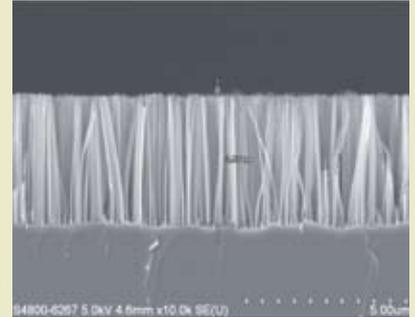
Silicon nanowire developed on silicon substrate for solar cell applications.
