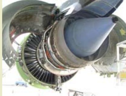
A typical jet engine mounted on an airliner.
