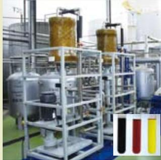
Vibratory membrane recycling system for used oil. The small photo shows oil at different filtering stages. (Courtesy of Dunwell Group)
