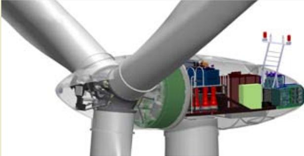
Wind turbine is a complicated electromechanical system. Its plant room typically houses servo control systems (to align the rotor axis with the wind and to give the blades the optimal angle of attack), gearbox, electric generator and power converter (to interface with the transmission network). (Courtesy of Avantis HK).
