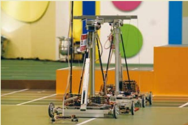
Robots designed and built by students for Asia-Pacific Robot Contest, consisting of microprocessor control boards, optical sensors, laser range finder, d.c. motors, motor drive boards and steering system.
